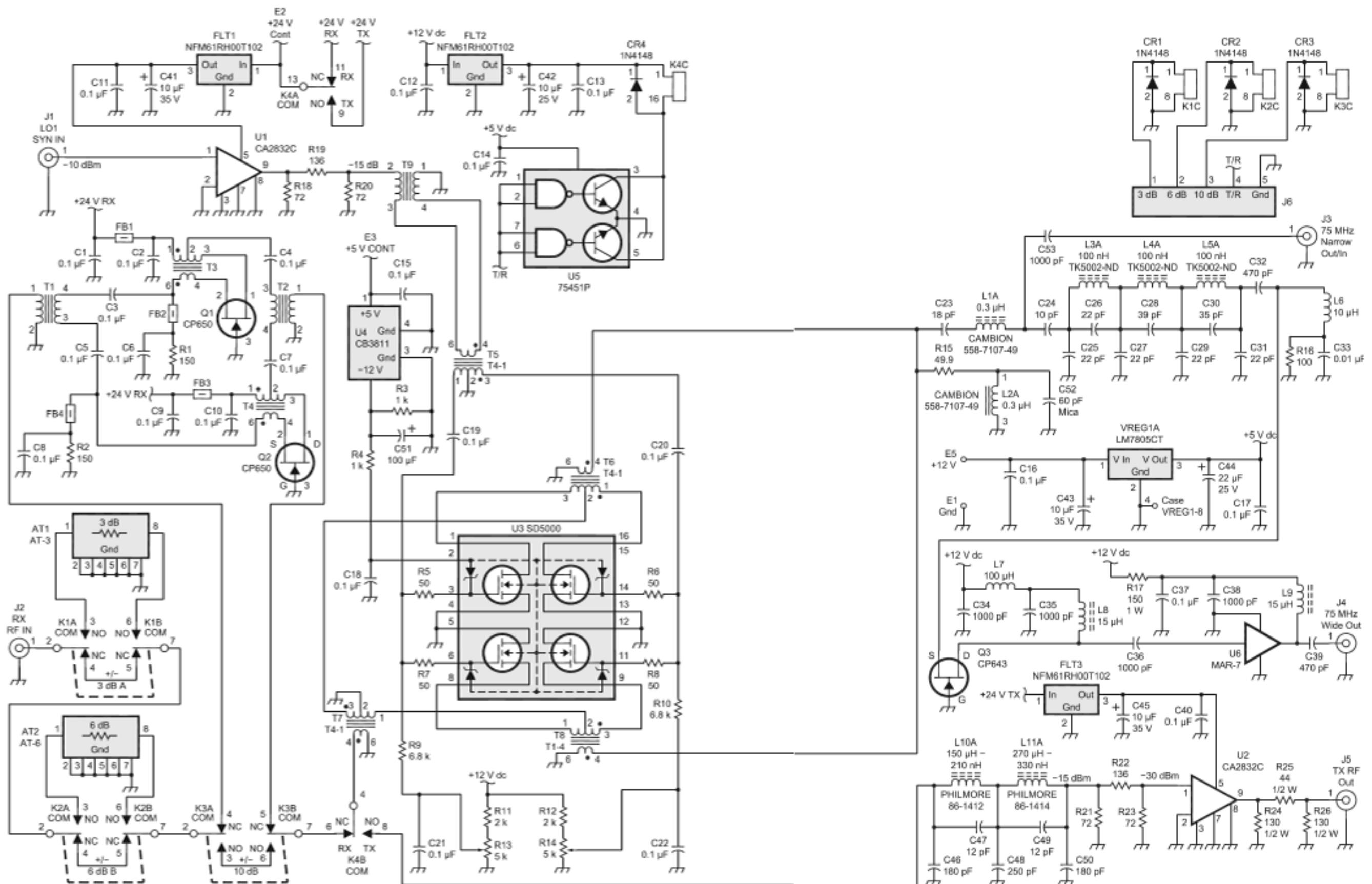
**Figure 14.1** Schematic diagram of the front end (upconverter, IF75BC) for the Star-10 transceiver. The receiver uses a push-pull Norton amplifier, a high-level H-mode mixer, and class A amplifiers. An MDS of  $-132$  dBm was calculated ( $-136$  dBm actual was measured) and an IP3 of  $+45$  dBm was predicted and found. Power consumption is over 30 watts DC. (From: [1-3]. Figure courtesy of ARRL.)
